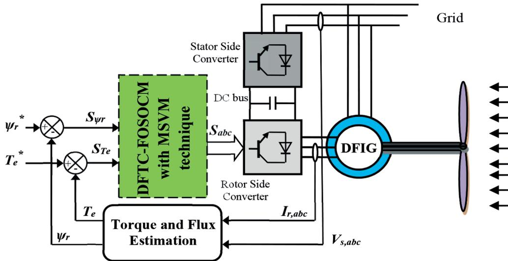
Figure 3. Block diagram of the DFIG with DFTC-FOSOCM
