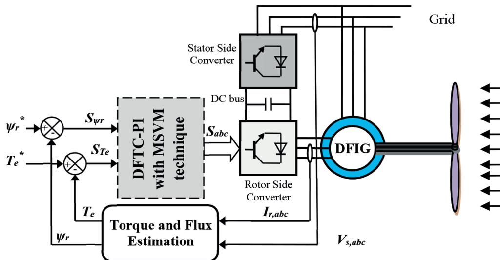
Figure 2. Block diagram of the DFIG with DFTC–MSVM
