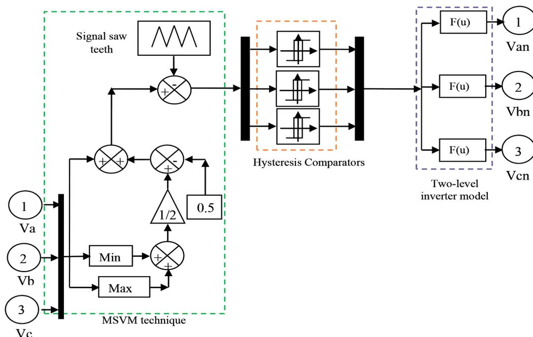
Figure 1. Block diagram of the modified SVM technique [41]
