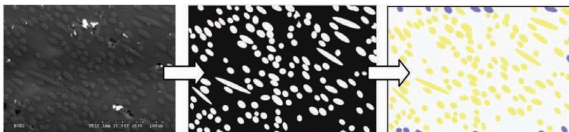
Fig. 5. Counting of carbon fibers in the surface layer of the composite (counting method)
