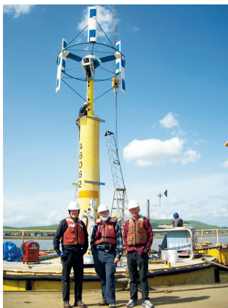
Fig. 1. Small 3 kW buoy based vertical axis wind turbine developed by the author team
